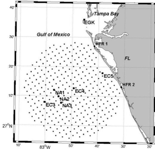
Fig. 1. Map showing coverage grid of the HF Radar, the two Radar sites (HFR1 and HFR2), the location of Egmont Key wind (EGK), and the USF ADCP mooring locations, including EC4 used in this study.
