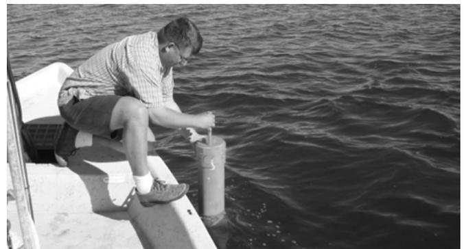
Fig. 5. Initial testing of the prototype drifter. For this version 1.6-cm (4-in.) PVC pipe was used. Since then everything has been shrunk to fit into a 1.2-cm (3-in.) PVC pipe with a longer and narrower antenna.
