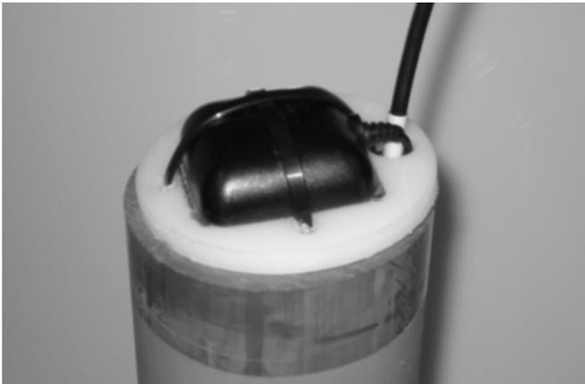
Fig. 2. Active GPS Antenna mounted on the top of the test drifter.
